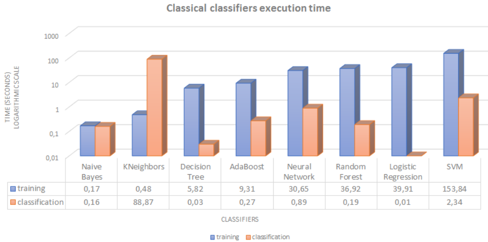
Figure 5.2: Training and classification time for classical classifiers (average for 10 folds). Pre-processing time is between 2 and 11 seconds
