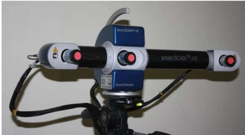
Figure 2 - Breuckmann SmartSCAN 3D Scanner. Image taken from (Santos, 2014).
