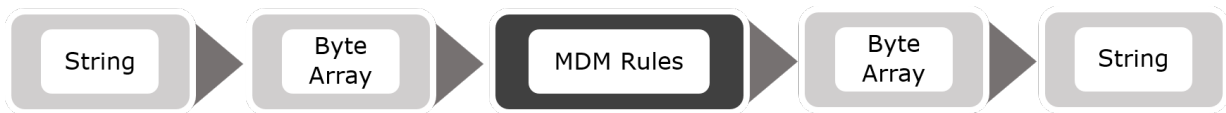
Figure 4.2: Visual representation of what happens when storing a string to apply cleansing or matching rules.
