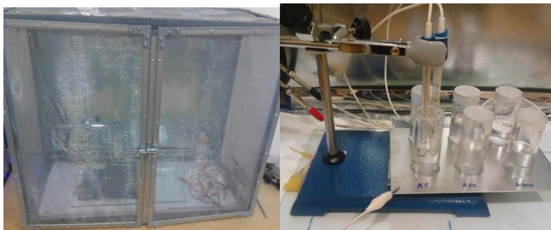
Figure 9: Faraday cage (left) and experimental installation (right).
