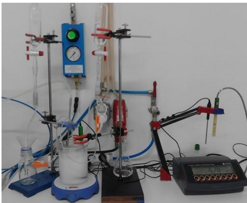
Figure 7: Experimental installation for the LDH synthesis.
