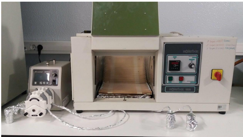
Figure 6- Scheme of SMX photodegradation in continuous flow mode.
