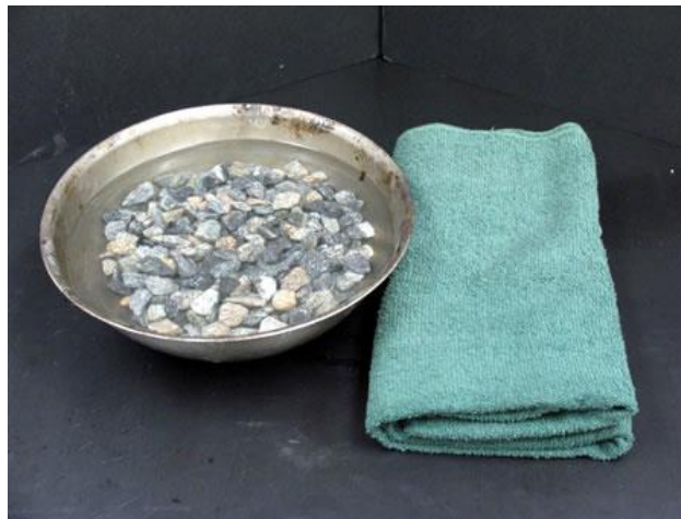
Figure 3.3.4- Coarse Aggregate Specific Gravity, pavementinteractive.org
