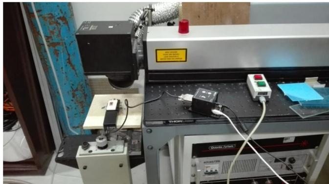
**Fig. 3.5:** Laser Nd-YAG (1064 nm).
