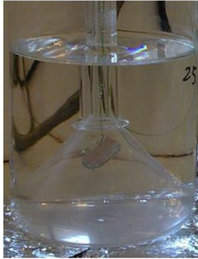
Figure II.8 - Illustration of a typical fishing line specimen under HE measurements. This method was used in the investigation work and the image is adapted from [114].
