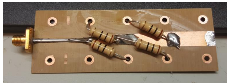
Figure 18 – 2.5 \Omega test load, used for high peak power tests.
