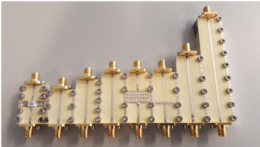
Figure 43 – TRL Calibration Kit used to measure packaged devices.
