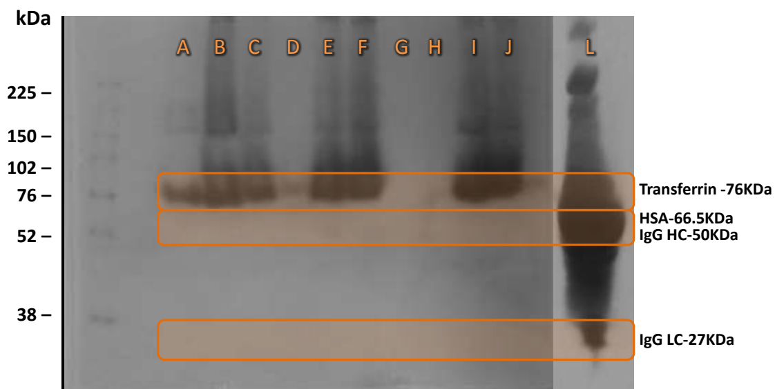
Figure 3.1.7. SDS-PAGE of proteins on IL-rich phase of the ABS composed of (a) [\text{MepyrNC}_4]\text{Br} (b) [\text{Et}_3\text{NC}_4]\text{Br} , (c) [\text{Pr}_3\text{NC}_4]\text{Br} , (d) [\text{Bu}_3\text{NC}_4]\text{Br} , (e) [\text{Pr}_3\text{NC}_4][\text{Lac}] , (f) [\text{Pr}_3\text{NC}_4][\text{Pyr}] , (g) [\text{Pr}_3\text{NC}_4][\text{Sac}] , (h) [\text{Pr}_3\text{NC}_4][\text{Dca}] , (i) [\text{Pr}_3\text{NC}_4][\text{Sal}] , (j) [\text{Pr}_3\text{NC}_2][\text{Sal}] and (L) human serum in PBS (1:10 (v:v, human serum)).
