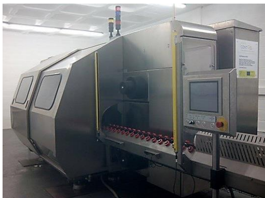
Figure 3.5 - CIP system used: U33 high pressure system from Unipress Equipment.
