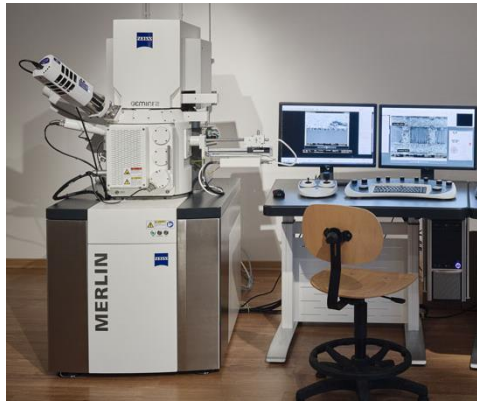
Figure 3.12 - FDSEM used for observation of the samples microstructure: ZEISS MERLIN Compact/VPCompact, present in IPN, Coimbra.
