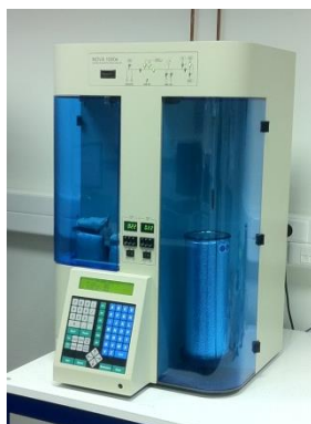
Figure 3.9 - SSA equipment used: Nova 1000e Series System, from Quantachrome present in INNOVNANO.
