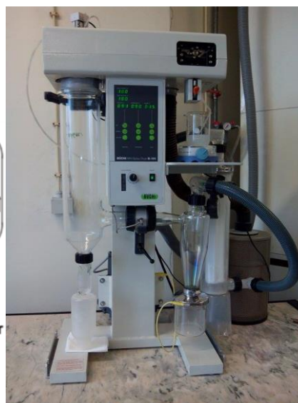
Figure 3.4 - Left: Schematics of the spray drying process from [115]; Right: Laboratorial Büchi Mini Spray-dryer B-191 used.
