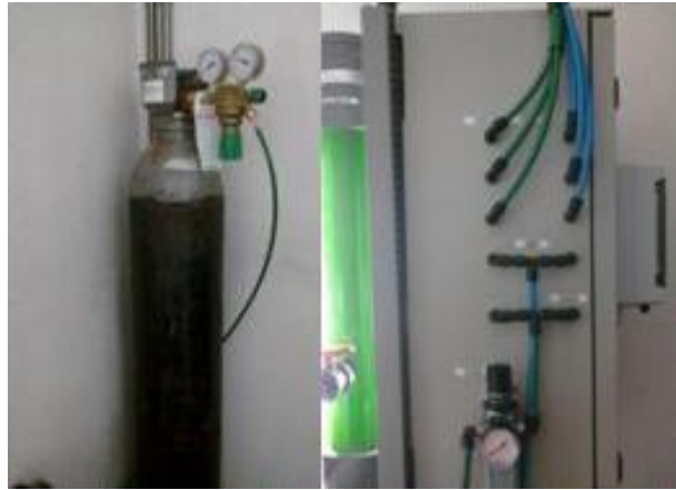
Figure 4-5 Left: CO 2 bottle, Right: CO 2 and air mixed and aerated to the culture. Green tubes: CO 2 , Blue tubes: Air (Photo credits: Smritikana Dutta)
