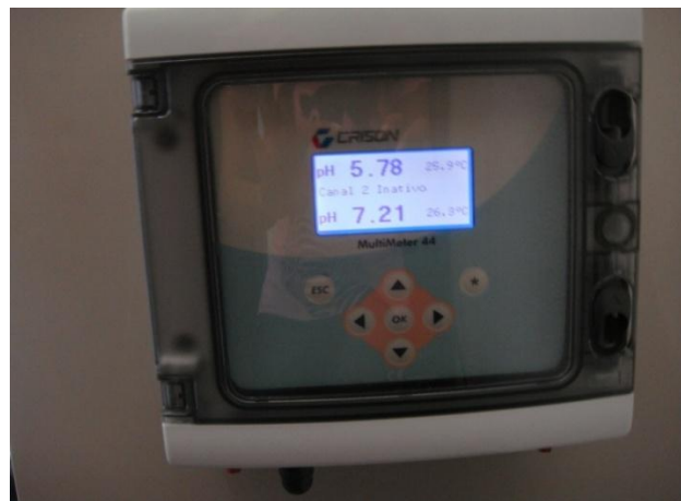
Figure 4-4 Multi-meter connected to the PBR to maintain the pH level of the culture (Photo credits: Smritikana Dutta)
