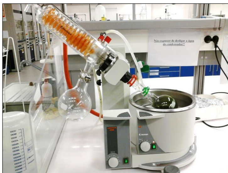
Figure 5-9 Chemical solvent hexane recovery after microalgae lipid extraction (Photocredit: Smritikana Dutta, University of Aveiro)
