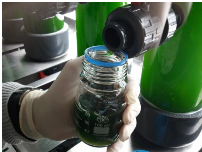
Figure 4-8 Collection of sample to measure daily cell growth (Photo credits: Smritikana Dutta)
