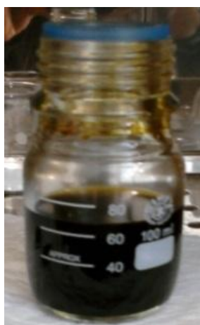
Figure 5-4 Pure biodiesel extracted from microalgae in Aveiro (Photo credits: Smritikana Dutta, University of Aveiro)
