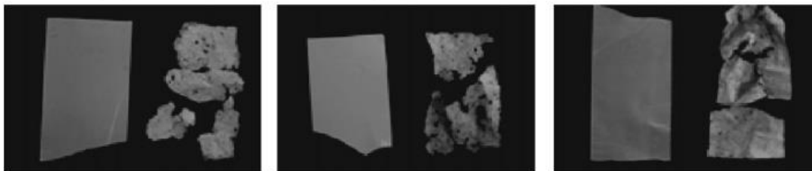
FIGURE 5 - Physical degradation of PHA films from mixed culture after 15.9 weeks of incubation (Arcos-Hernandez et al. 2012).
