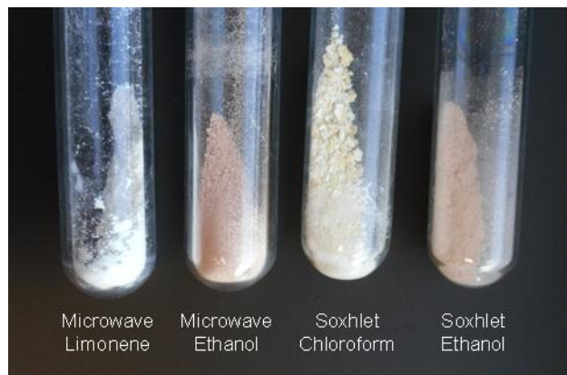
Fig. 3 Birch outer bark extracts obtained by Soxhlet and microwave assisted extractions. The extraction method and the used solvent are indicated in the figure.
