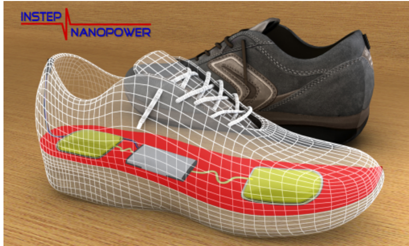
Figure 3.7: Energy harvester human motion concept. src: Krupenkin, T. & Taylor, J. A. - kurzweilai.net
