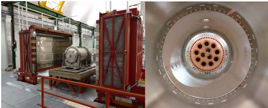
Figure 2.9: NEXT NEW TPC installed at LSC (Canfranc, Spain) and detail of the vessel interior showing the PMTs copper enclosures.
