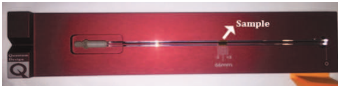
Figure 3.20: Thin film sample mounted for magnetization measurements.
