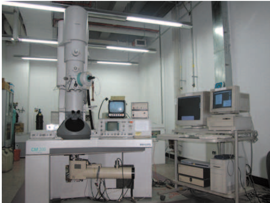
Figure 3.16: Philips CM200 FEG microscope, used in thesis, FHI, Berlin.
