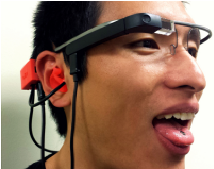
Figure 2.10: Tongue magnetometer and Outer Ear Interface [Sahni et al., 2014].
