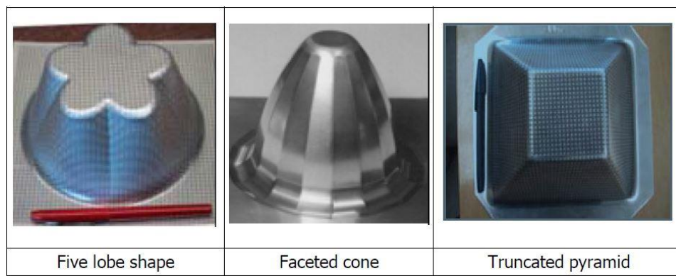
Figure 11: Examples of geometries produced by SPIF (Jesweit 2005) (M. Martins 2011).
