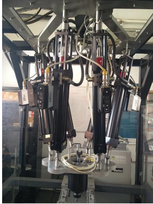
Figure 31: SPIF machine used in this work.
