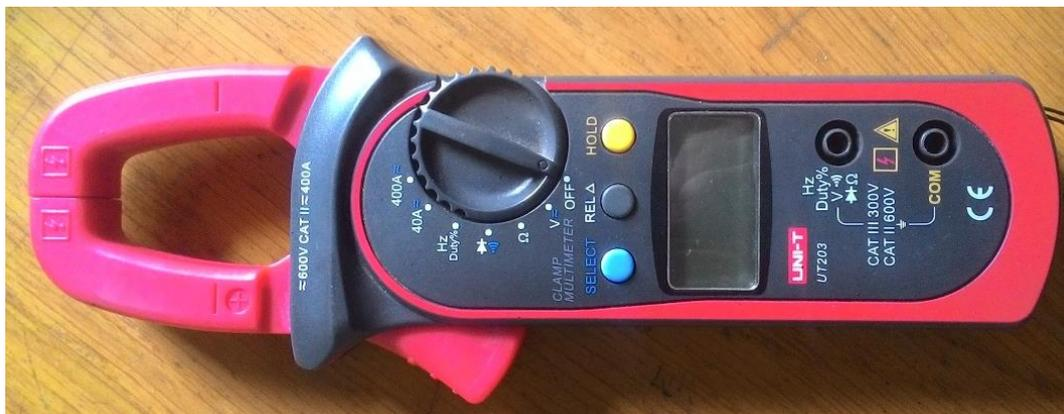
**Figura 19 – Pinça digital (digital clamp multimeters)**
