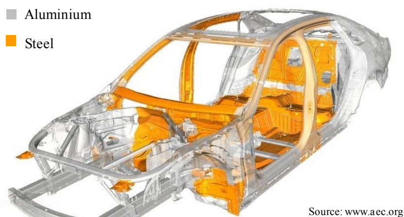
Figure 1-1 Cadillac CT6 mixed material lightweight structure.
