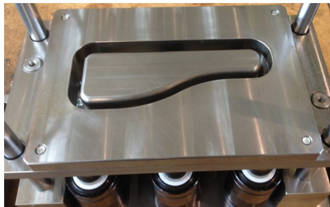
Figure 5-9 Experimental lower die set with punch for P-channel.
