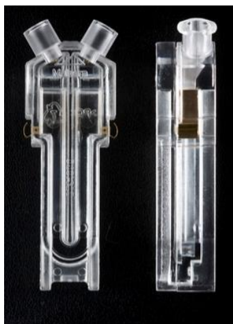
Figure 18: Disposable folded capillary cell for measurement of zeta potential (source: LabBulletin, 2009)
