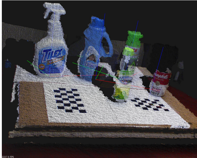
Figure 1.1: Point cloud captured by a robot: example of what a robot can perceive from the world using vision systems.
