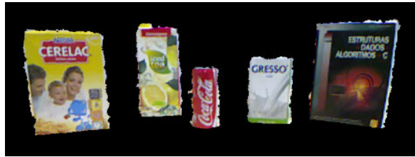
Figure 3.12: Screenshot of the set of point clouds resulting from the clustering process.
