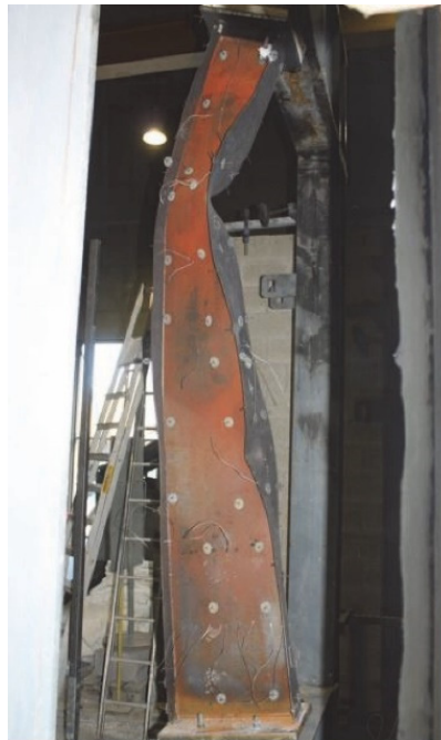
Figure 3.2: Example of column showing local buckling from a test performed at elevated temperatures at the University of Liège (taken from[3.13]).
