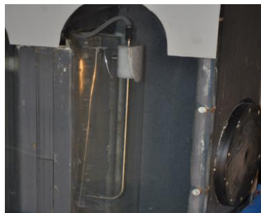
b) TSS nozzle placed inside the tank.
