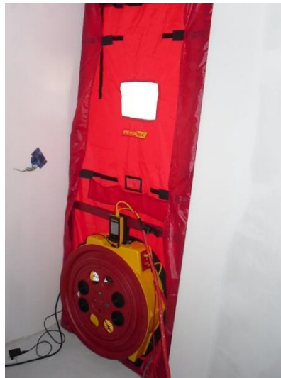
Figure 42 – Blower door installed to conduct the experiment.
