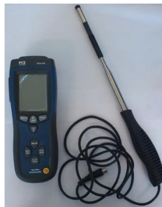
Figure 41 – Digital anemometer used to register air velocities in experimental procedure 1.
