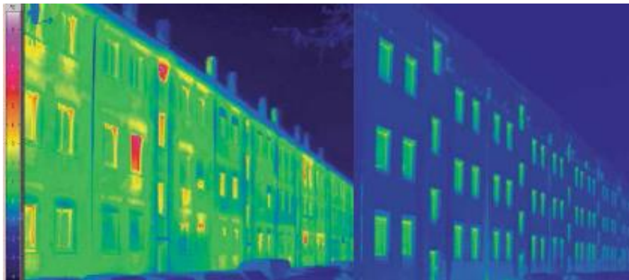
Figure 3 – Thermographic image showing the advantages of a proper thermal insulation (adapted from IPHA, 2014).
