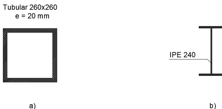
Figura 4.8- Perfis transversais, a) tubular 260x260, b) IPE 240.
