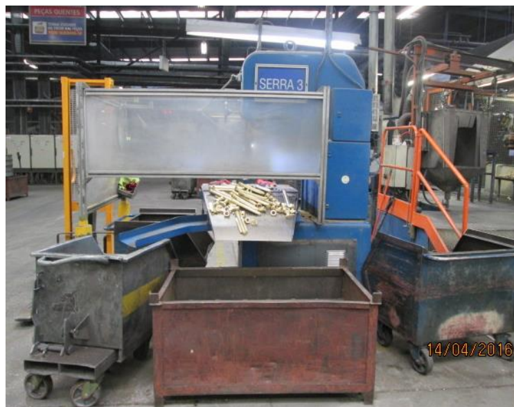
Fig. 6 - Band saw for gating system and piece cutting.
