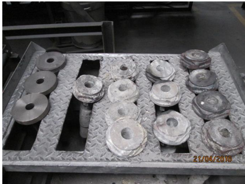
Fig. 25 - New riser tubes (first row) and used riser tubes (right side).
