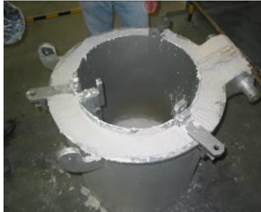
Fig. 4 - Distribution ladle for transportation and distribution of the liquid brass to the casting machines.
