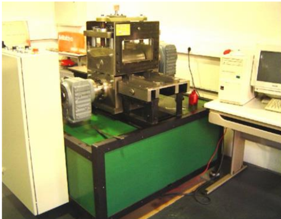
Figure 3.11 - Asymmetric rolling machine available at University of Aveiro.
