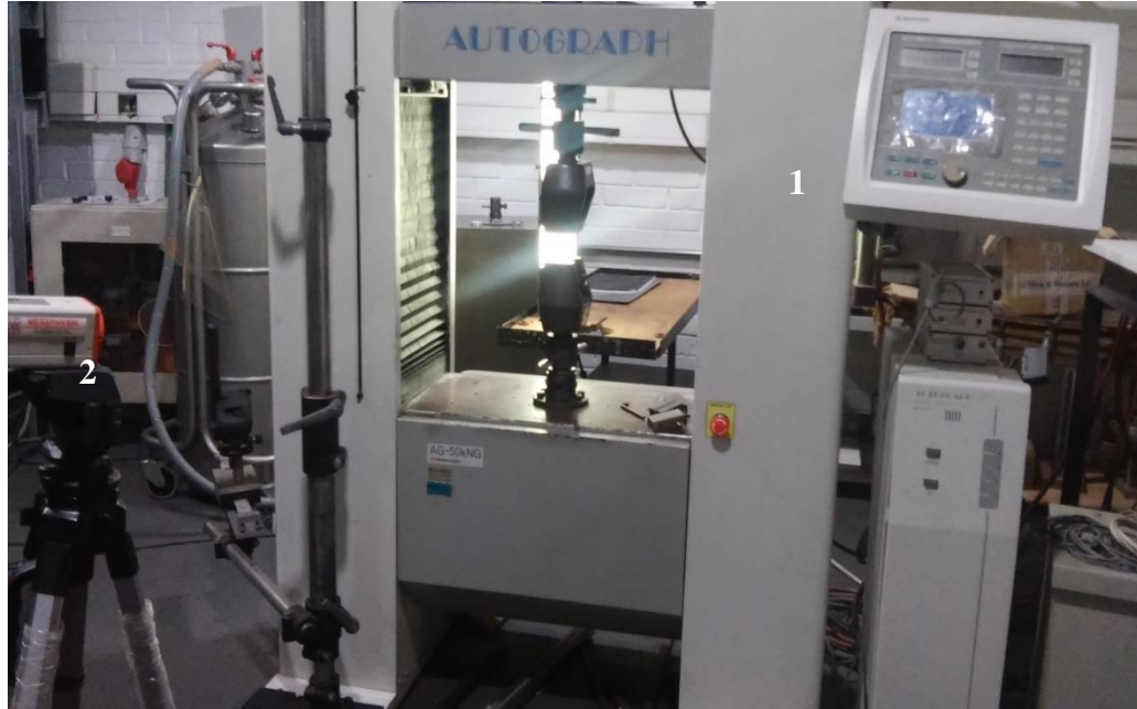
Figure 3.7 - Tensile Test Equipment used in this study: 1 - Shimadzu Autograph Machine, 2 — video extensometer.
