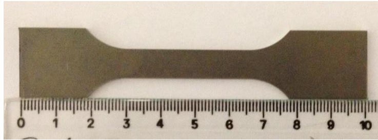
Figure 3.9 – TWIP steel specimens shape used for tensile test
