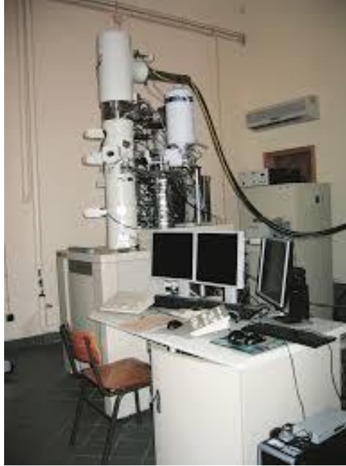
Figure 3.14 - JEOL 2200FS High-Resolution Energy-Filtered Transmission Electron Microscope available at University of Aveiro.
