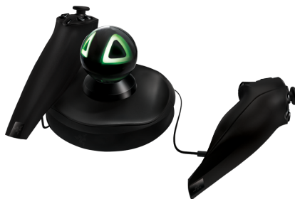
Figure 2.18: Razer Hydra magnetic tracker
