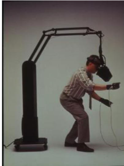
Figure 2.19: BOOM Display (Craig, Sherman, and Will, 2009)
