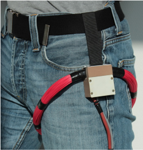
Fig. 3. The primary power coil around a patient's hip (Bergmann et al., 2012). Having a coil around the hip is uncomfortable and troubles the activities of the patients.
