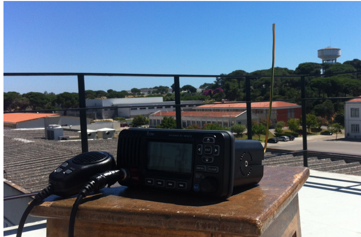
Figure 6.28: Maritime VHF radio with short wire acting as an antenna, for transmitting power control.
