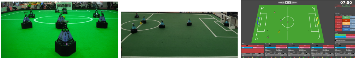
Figure 1.4: On the left and center images, an example of a robot setup during a soccer game. On the right, the world as the robot understands it, displayed on the team base-station.
