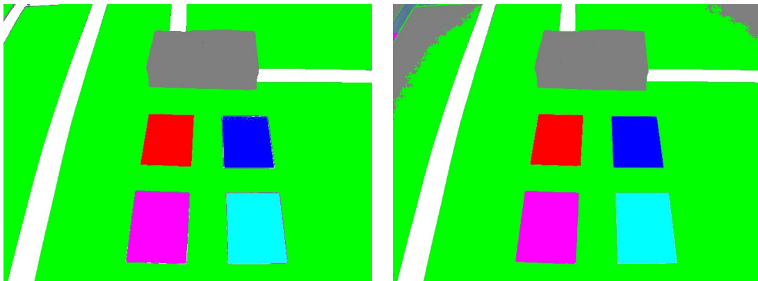
Figure 7.3: On the left, one of the images used as ground truth validation. On the right, the color classification performed by an user.
