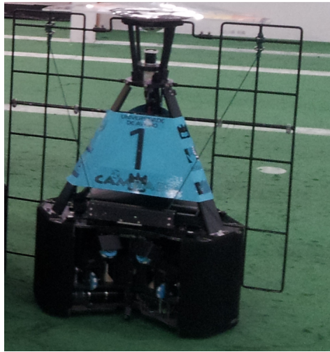
Figure 5.15: The goalie of the robotic soccer team CAMBADA with the Kinect sensor installed on its frontal part.
