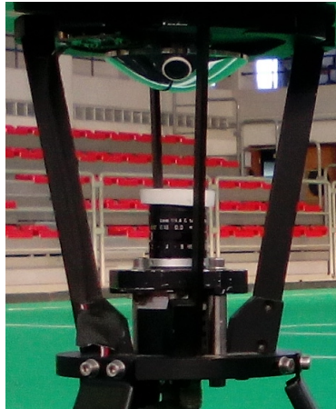
Figure 5.2: Mirror and digital camera disposal of the omni-directional vision system.
