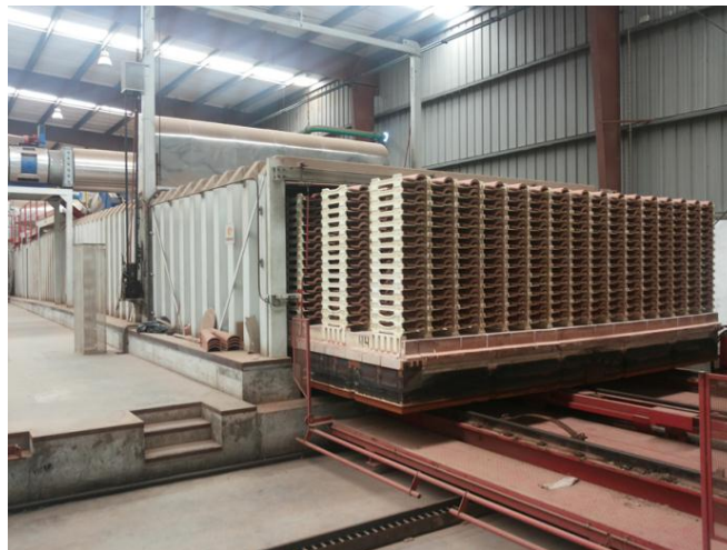
Figura 3.14 - Forno Ceric hydrocasing
