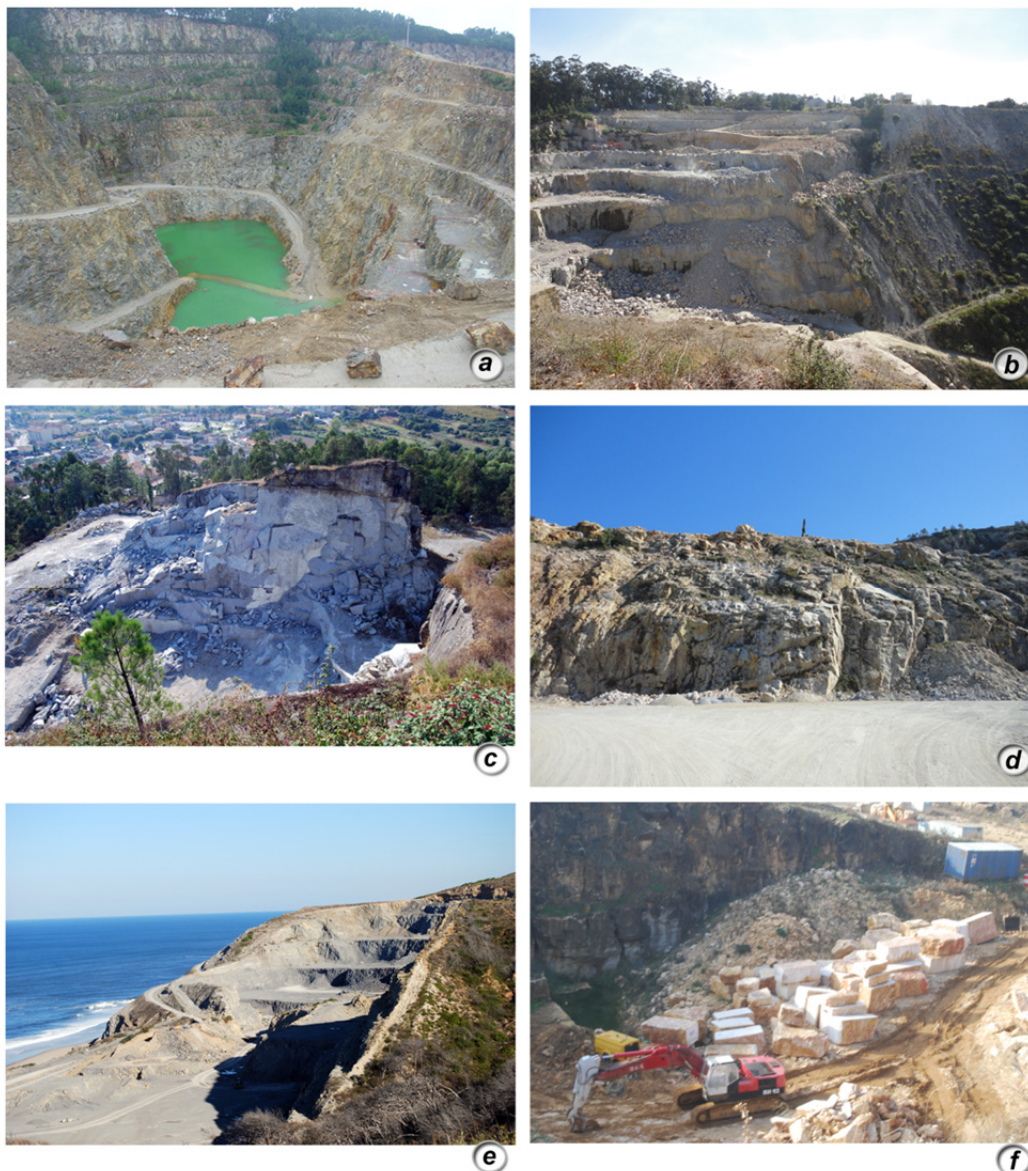
Figure 114. Type of rock quarries and some examples of the georesources available: (a) granite quarry for aggregate/armourstone (Malaposta quarry, S. João de Ver, NW Portugal); (b) granite quarry for aggregate/armourstone (Madalena quarry, Canidelo, Gaia, NW Portugal); (c) granite quarry for ornamental rock (Bouça dos Castros quarry, Braga, NW Portugal); (d) granite quarry for aggregate (Vilar quarry, Ribeira, NW Galicia); (e) limestone quarry for aggregate (Cabo Mondego Norte, Figueira da Foz, Centre Portugal); and (f) limestone quarry for ornamental rock (Alenquer quarry, Lisbon, Central Portugal); (Photo credits: A. Pires and J. Teixeira).
