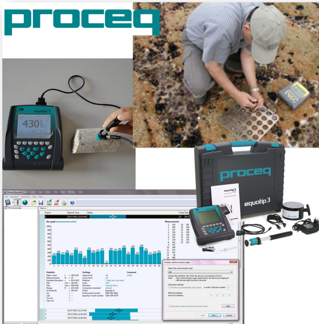
Figure 42. Proceq's Equotip equipment general overview and the interface of Equolink, the linking software.
