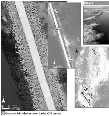
Figure 3. Example of mixed coast of Aguiño groyne with rocky platform: (a) and (b) general overview of the studied sector; (c) and (d) GIS mapping of all the geomaterials.
