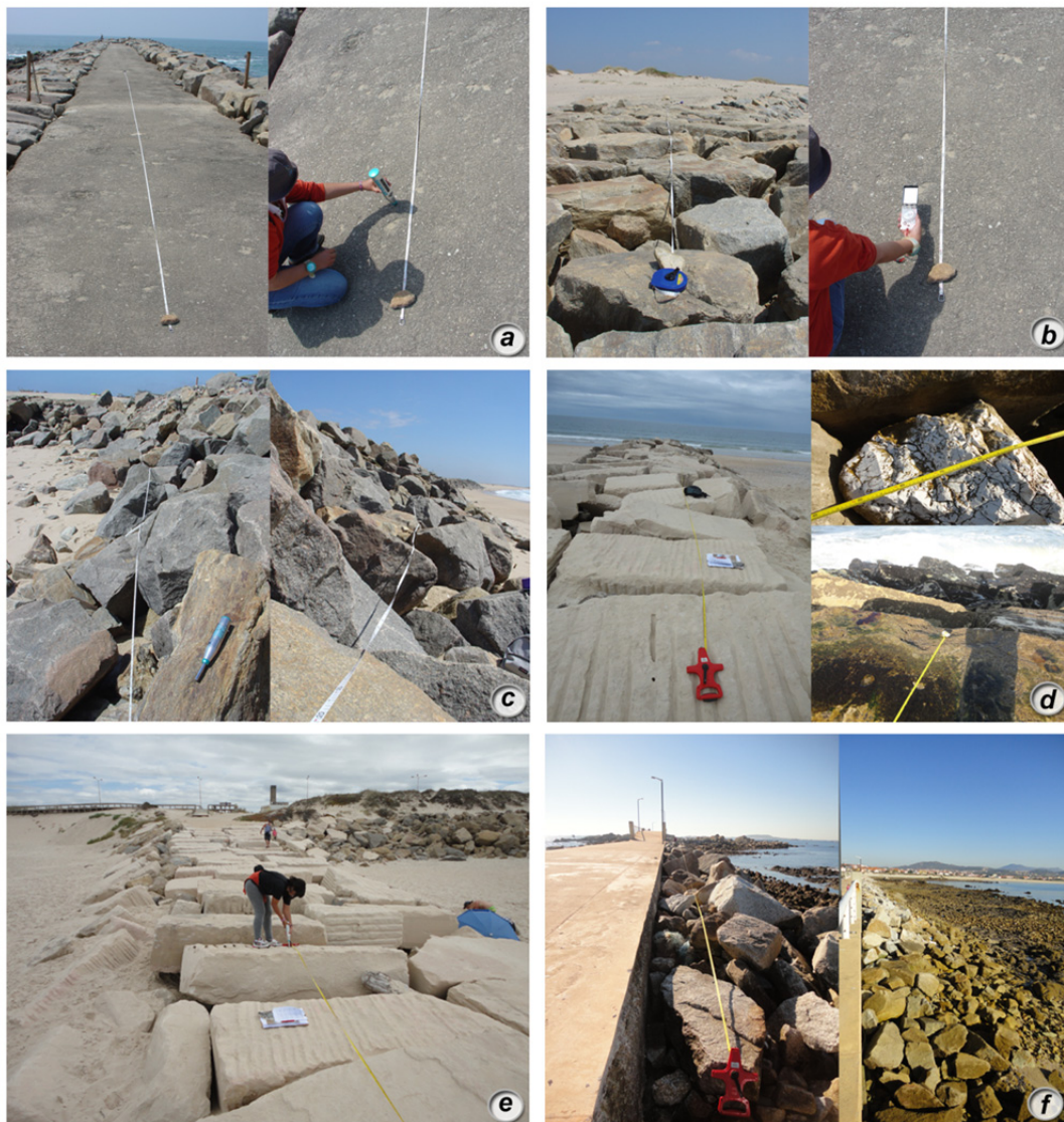
Figure 64. The scanline technique applied to maritime structures.
