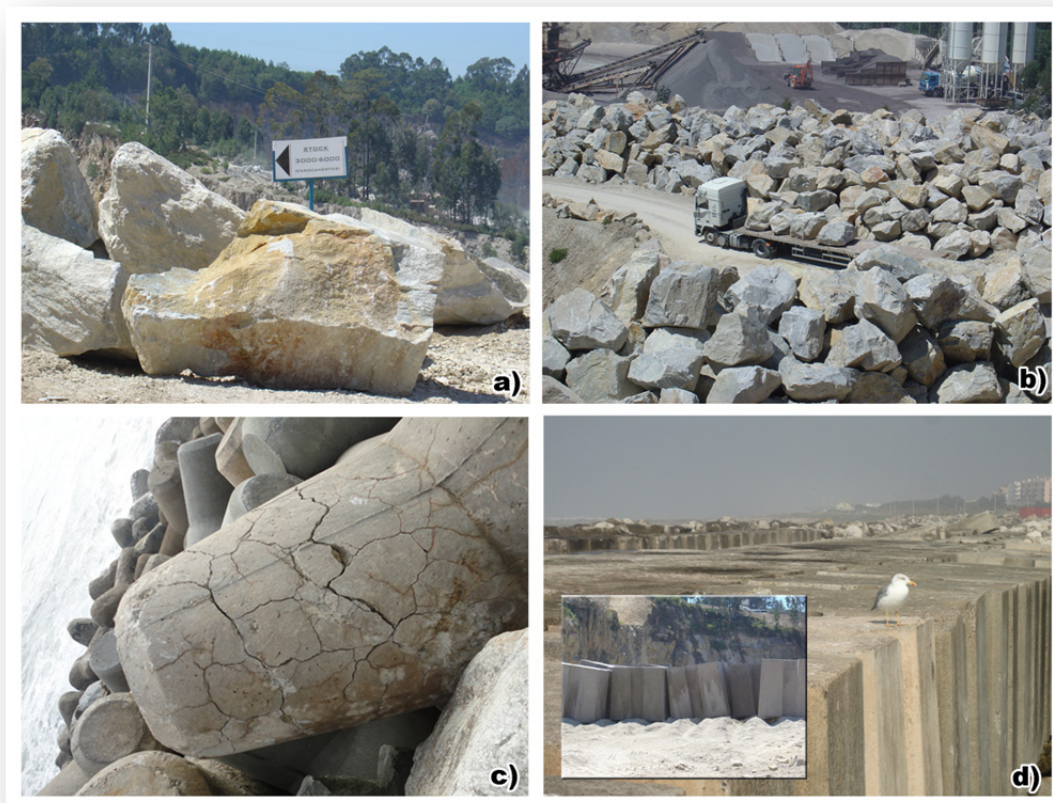
Figure 115. Types of geomaterials applied in marine structures: (a) and (b) armourstone (natural rock) and concrete armour units (artificial blocks): tetrapods (c) and antifers (d) (Photos by A. Pires).
