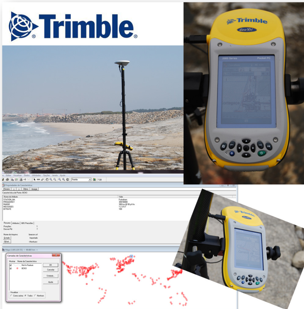
Figure 39. Trimble GPS model GeoXH™ incorporating the external antenna. Also displayed is the interface of the Trimble GPS Pathfinder® Office software, which is a powerful and accessible package of GNSS (Global Navigation Satellite System) postprocessing tools.
