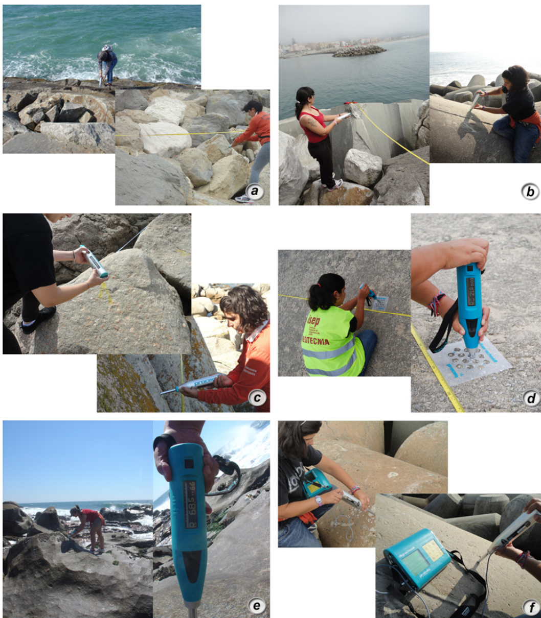
Figure 62. Several applications in situ of the Original Schmidt hammer, Silver Schmidt and Digi Schmidt at the studied sites.
