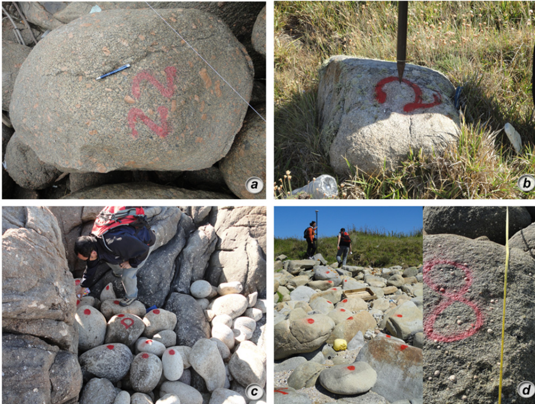
Figure 50. Boulder monitoring and systematic observation to trace the movement and displacement of blocks with markers (Laxe Brava, NW Galicia, Spain); visual inspection applied to rocky coasts and boulders beach.
