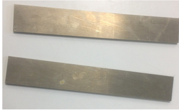
Figure 3.1: AA2024-T3 plates to be welded.
