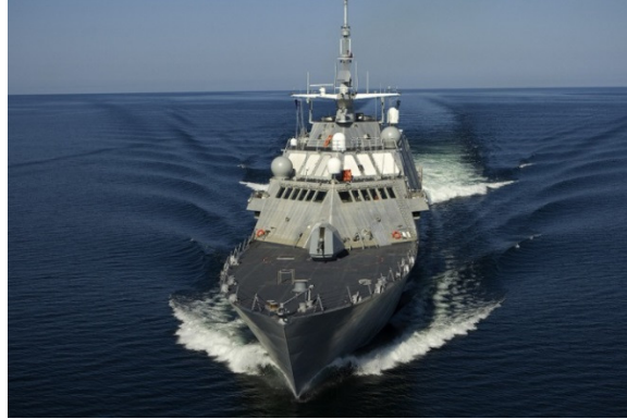
Figure 2.8: Littoral Combat Ship USS Freedom, built using FSW technology for aluminium alloy joining [10].
