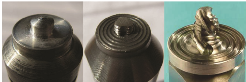
Figure 2.4: Different FSW tool designs [36].
