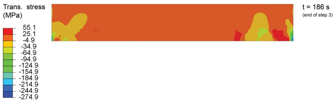
Figure 4.22: Stress results during the FSW analyses: (a) evolution of the magnitude of the longitudinal stresses, and (b) the transverse stresses at the end of the analysis.
