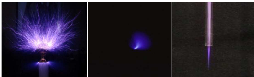
Figure 25 - Three types of Corona discharge. From left to right, Brush, Glow and Plume. [95, 102, 103]
