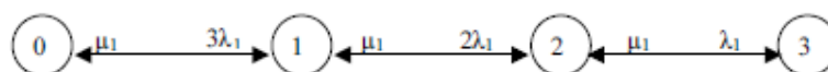
Fig.1 Markov graph for the subsystem of dialysis for infectious hepatitis B patients.
