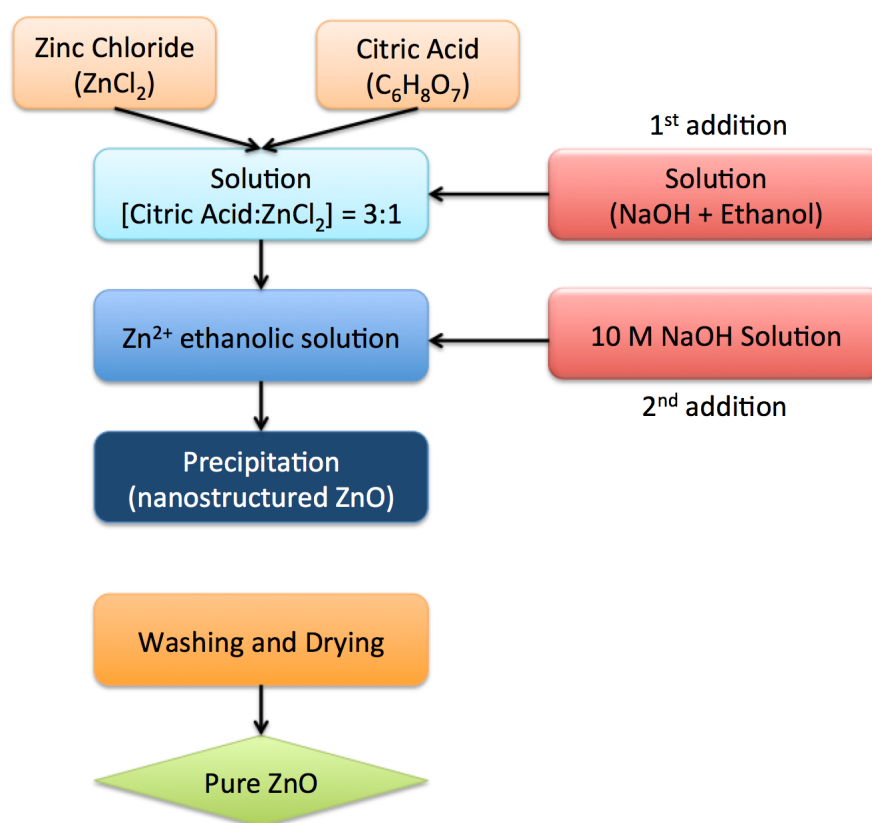
Figure 27: Flowchart outlining precipitation of nanostructured zinc oxide powder
