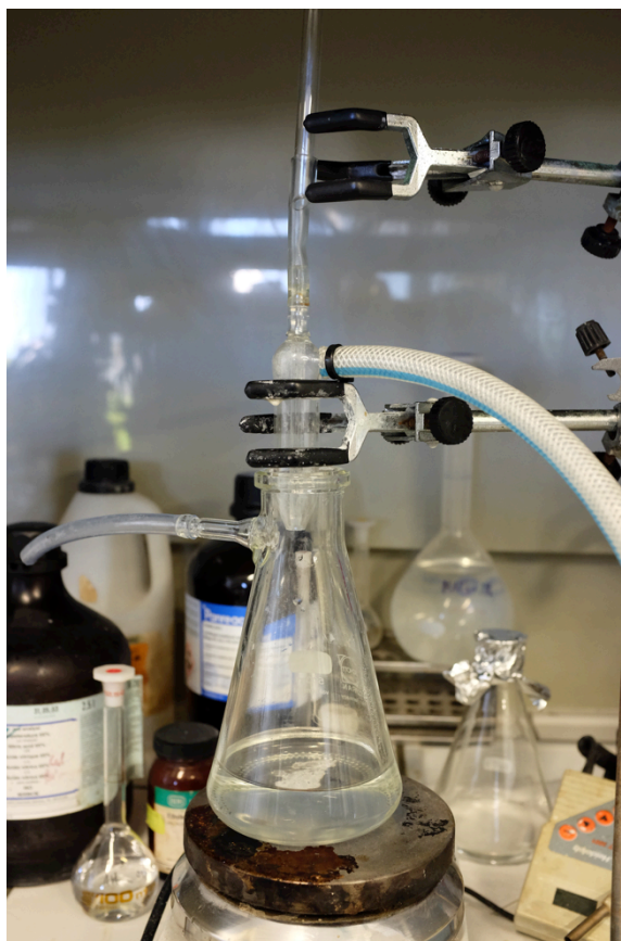
Figure 26: Setup of blowing apparatus for chemical precipitation of nanostructured zinc oxide
