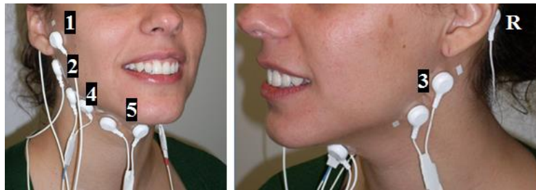
Figure 51. EMG electrode positioning and the respective channels (1 to 5) plus the reference electrode (R). EMG 1 and 2 use unipolar configurations whereas EMG 3, 4 and 5 use bipolar configurations.
