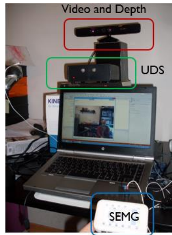
Figure 33. Setup A: Acquisition devices and laptop with the data collection application running for setup A based on (RGB) Video, Depth information (provided by infrared reflection), Ultrasonic Doppler sensing and Surface Electromyography.
