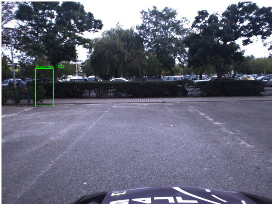
Figure 4.19: FP Fusion Algorithm Example - After a pedestrian passed the bushes, the classification continued to be shown for a short period of time
