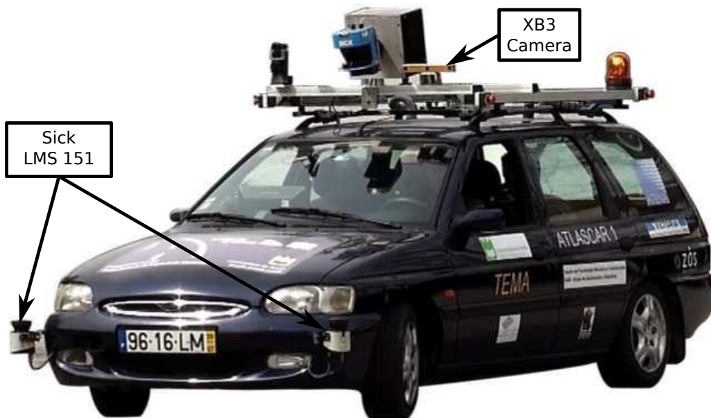
Figure 2.7: XB3 and Front Bumper laser localization in the car
