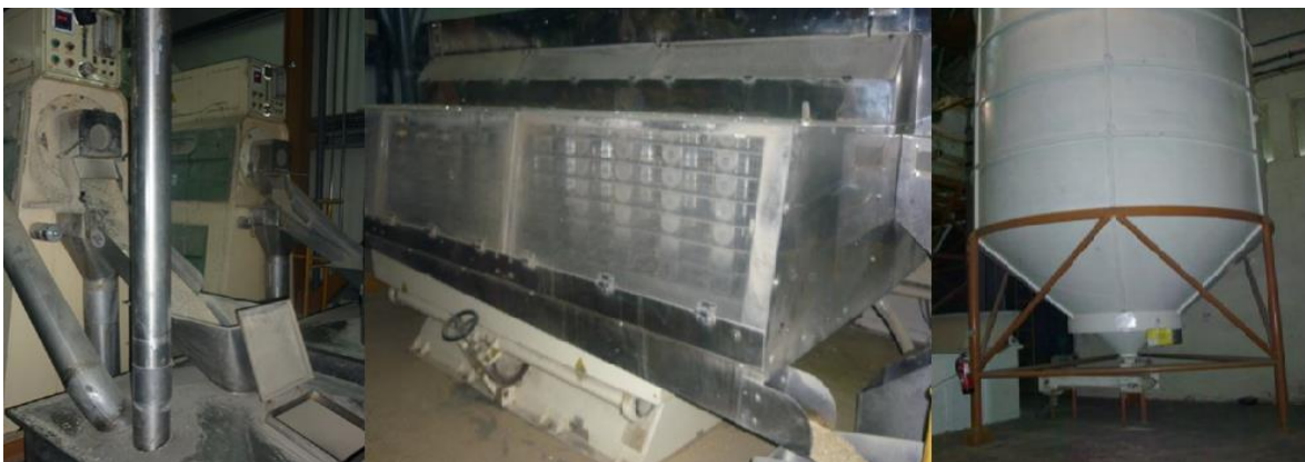
Figure 7 – Polisher (left), grade/sifter (centre) and silos of milled rice (right).
