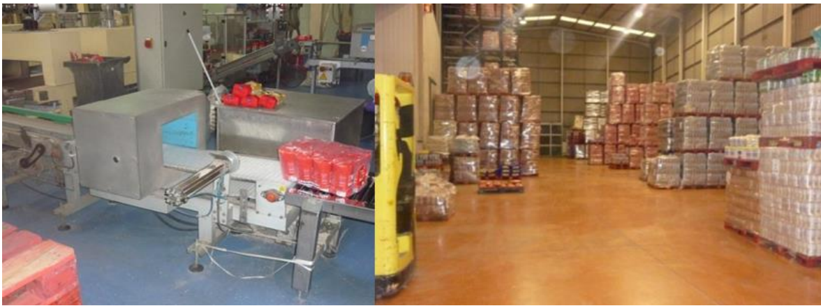
Figure 8 – Metal detectors at the end of the packaging line (left) and storage area for packaged goods (right).
