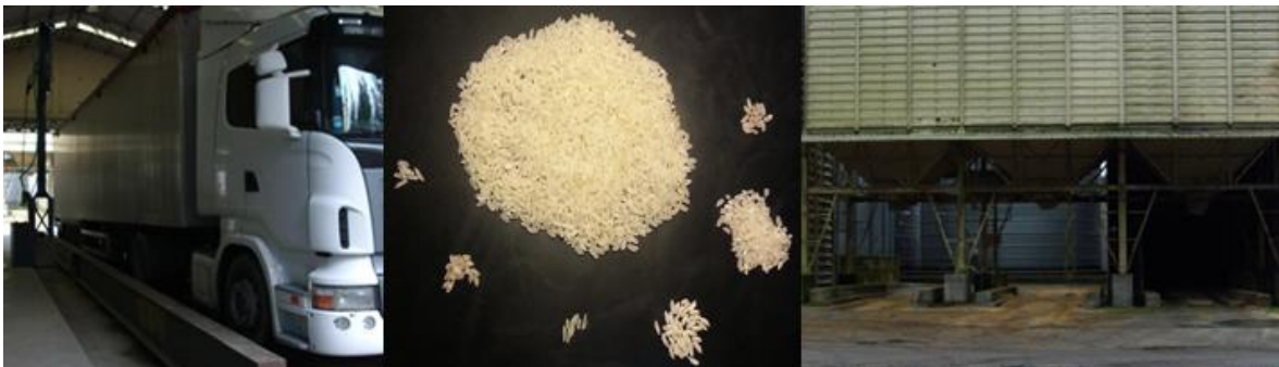
Figure 6 – Rice cargo being weighted (left), assessment of the percentages of impurities and defects (centre), and silos used for storage of the paddy rice cargo (right).
