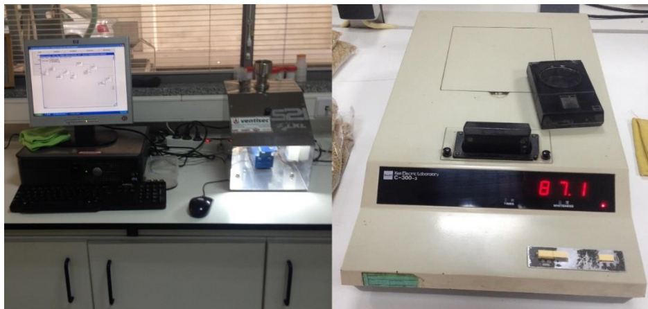
Figure 9 – AgroMay Statistic Analyzer S21 apparatus (left) and Kett Electric Laboratory, model C-300-3 apparatus (right).
