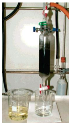
Figure 1.3.4: Experimental apparatus for decolorizing ionic liquids.
