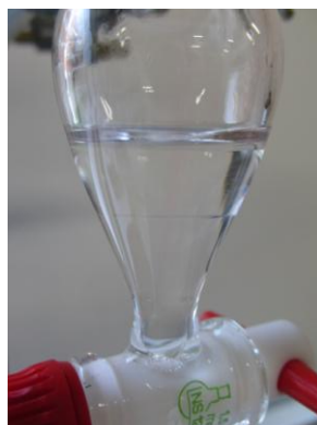
Figure 1.2.3: Macroscopic aspect of an ABS composed of PEG and an inorganic salt.
