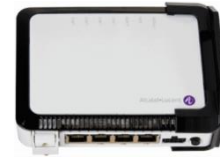
Figure 109 – Alcatel Optical network terminal. Source: http://www.alcatel-lucent.com/product .
