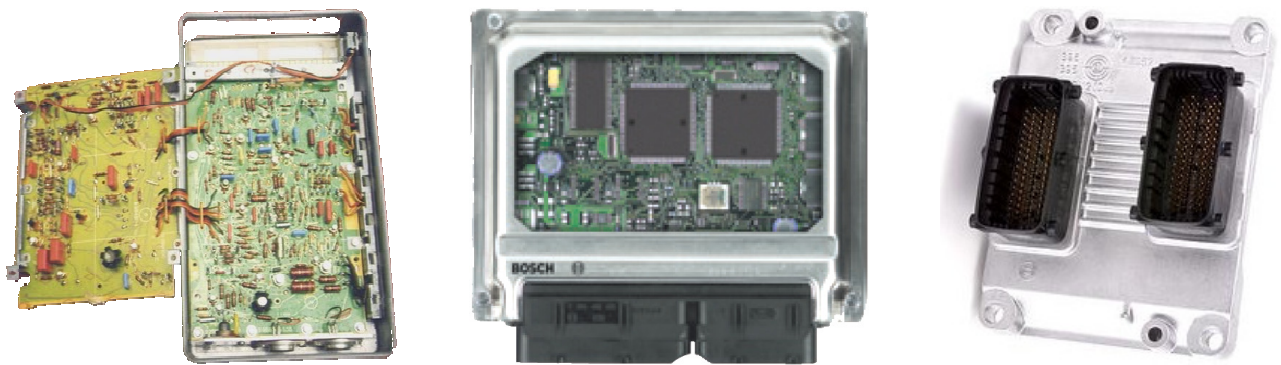
Fig. 2.2:50 – Older "D Jetronic", newer "ME7.1.1" & hybrid-technology "MS3" (source: Lucas & Bosch [93])
