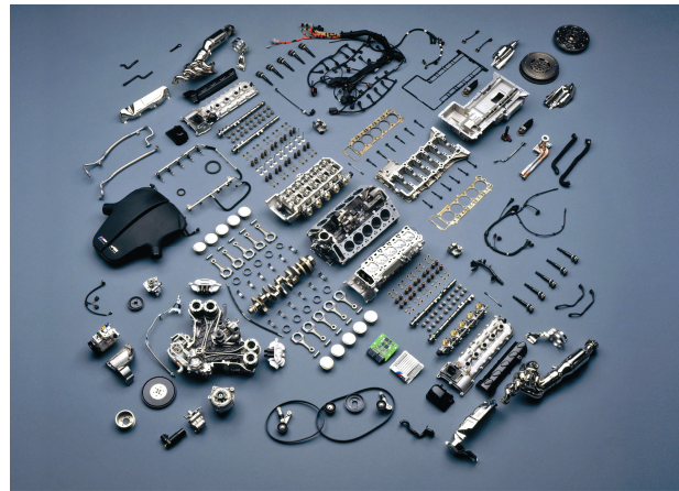
Fig. 1.2:4 – BMW “M” V10 engine with all its components (source: BMW)
