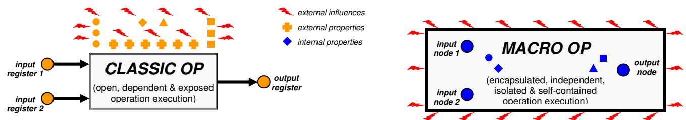
Fig. 4.2:10 – Comparison of classical exposed operation with the new shielded "Macro" operation
