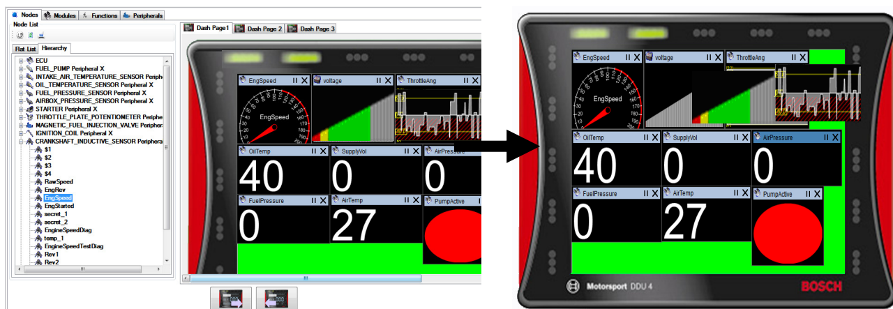
Fig. 5.1:25 – Seamless dashboard design through selecting "Nodes" at the right and the "race mode" viewing
