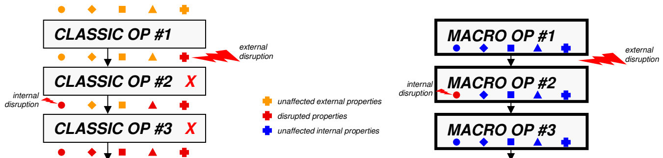
Fig. 4.2:11 – Comparison of bug propagation behaviours after an external and/or internal disruption
