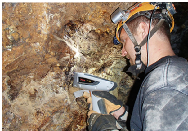
Figura 60 - Ensaio in situ com analisador FRX. ( http://www.burgex.com/services/ore-sampling/ , 2014)
