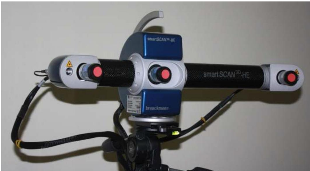
Figure 2 - Breuckmann 3D Scanner. Image taken from (Santos, 2013)
