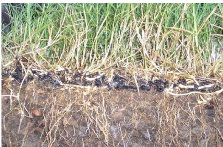
Figure 26. Vegetated high performance TRM system. Soil reinforcement is provided by the interlocking between the roots and mat (Hulitt, 2010).
