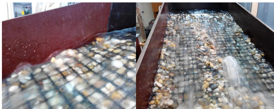
Figure 78. Waterflow depth profile (on the left picture) and water jet created due to irregularity of the surface granular layer (on the right picture).
