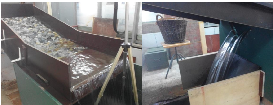
Figure 47. Sediment trap (hydraulic model's horizontal platform) releasing water to the container (on the left picture). Detail of v-notch weir installed in back part of the container (on the right picture).
