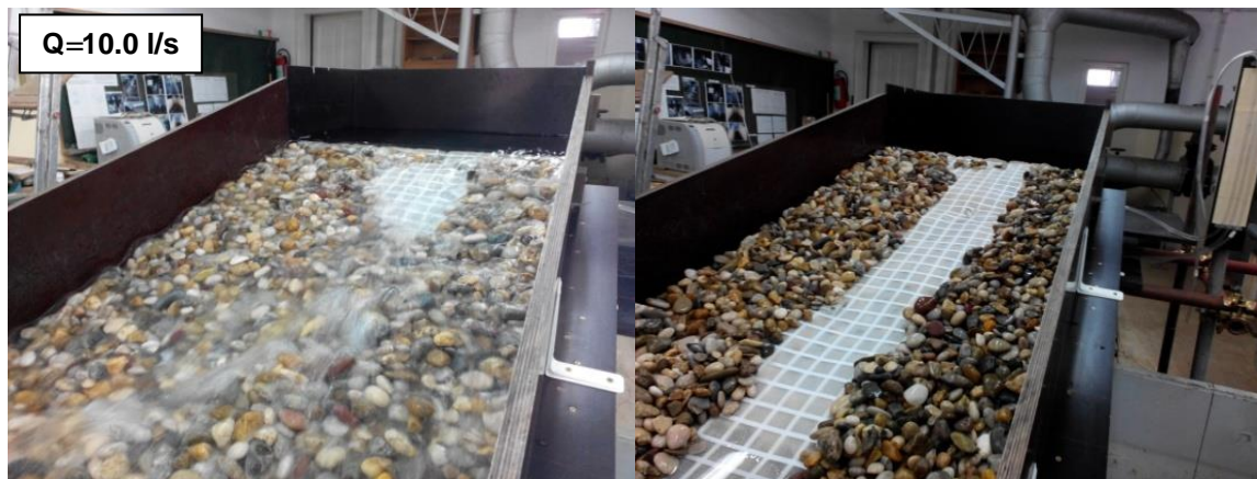
Figure 67. Development of a breach channel above the RECP M_2 .
