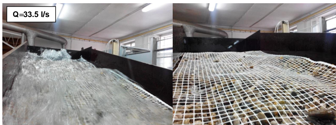
Figure 73. Bed channel being submitted to Q_{max} (on the left picture). Bed channel configuration after overtopping event has been ended (on the right picture).
