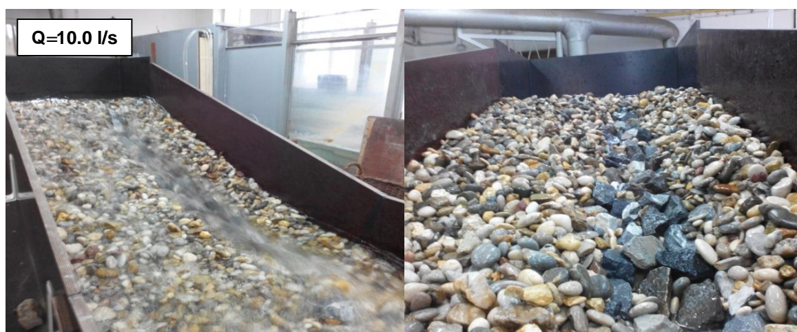
Figure 64. Formation of breach channel through the slope's granular revetment.
