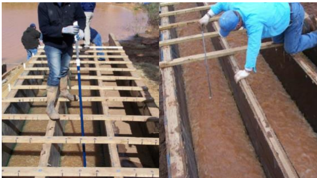
Figure 33. Flow velocity measurement (on the left picture) and flow depth measurement (on the right picture) in the testing channel (Nelsen, 2005).
