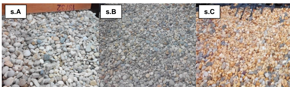
Figure 52. Coarse-grained soil samples for overtopping tests.
