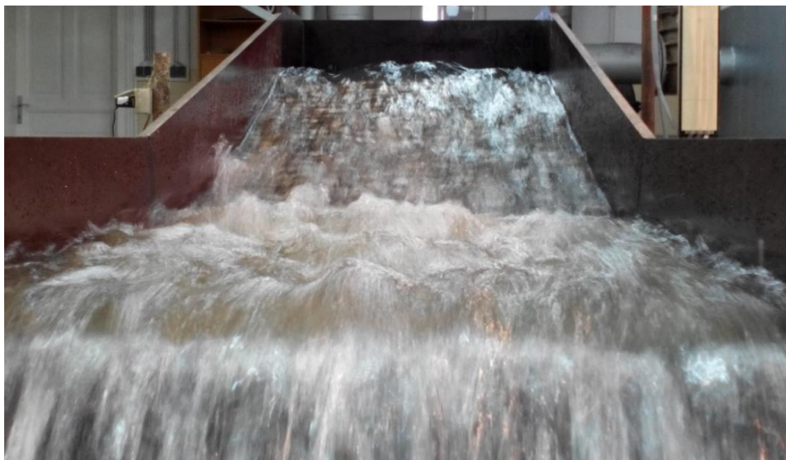
Figure 77. Flowing water exhibiting turbulence ( Q_{max}=29.6 l/s).
