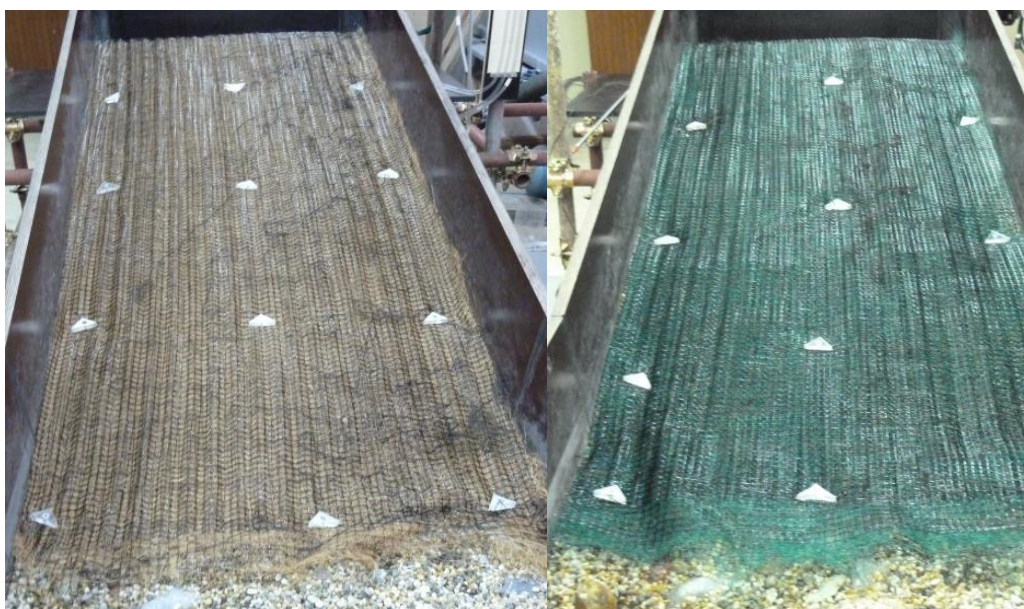
Figure 57. RECP M 5 (Vmax C350 ® ) (on the left picture) and RECP M 6 (Vmax C350 ® ) (on right the picture) with anchorage density of 8.2 anchors/m 2 over the channel slope.
