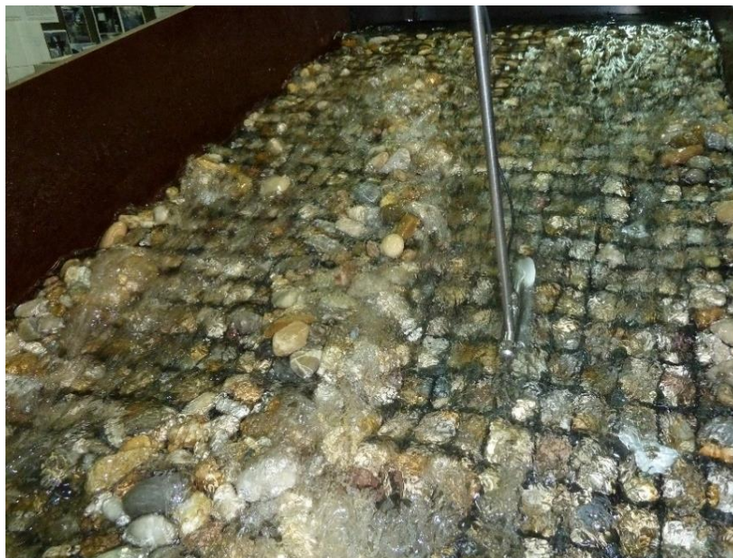
Figure 76. Measurement of velocity with an unsubmerged velocimeter.
