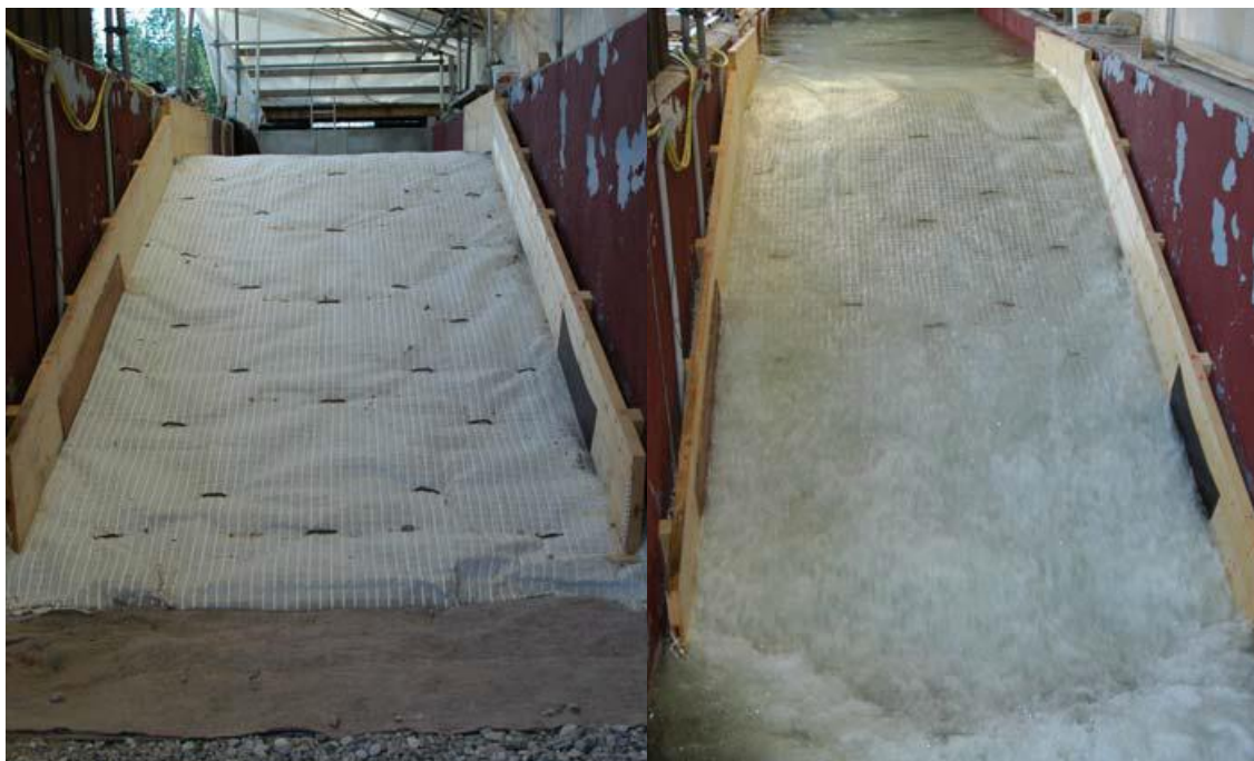
Figure 36. Overflowing experiments with a slope protection system with geosynthetics (Combigrid ® ). On the left: before overflow; on the right: in overflow state with q_{max}=300 l/s/m (Haselsteinaer et al. , 2008).
