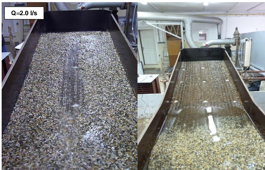
Figure 74. Initiation of the erosion process at the gravel top layer (beneath the TRM M 5 ) (on the left picture). Bed channel configuration after the overtopping event has ended, i.e. , after Q_{max} (on the right picture).
