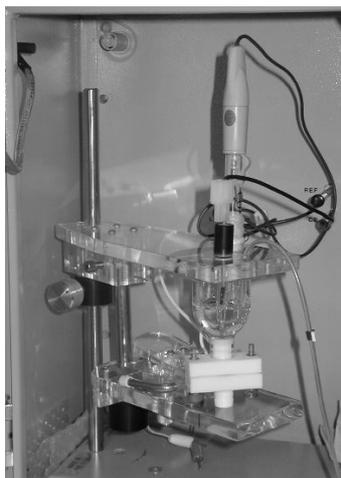
**Figure 2:** Experimental layout (electrochemical quartz crystal microbalance and cell with the three electrodes).
