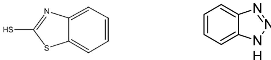
Figure 3 – Schematic presentation of 2-mercaptobenzothiazole (a) and 1,2,3-benzotriazole (b) molecules.
