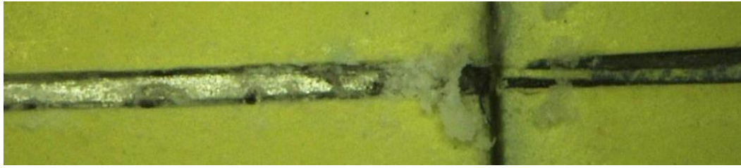
Figure 61 - General view of the AA2024 sample after 48 hours in SST
